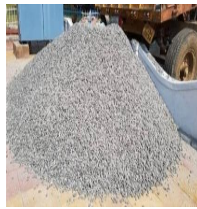
Value added products (Aggregates) from fly ash at RSTPS)
