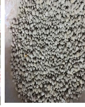
Value added products (Aggregates) from fly ash at RSTPS)
